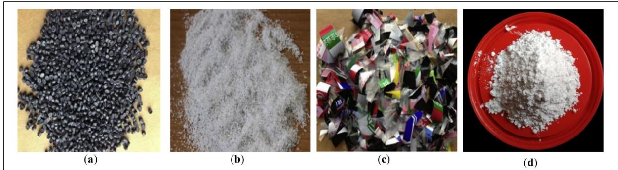
Figure 2 Various forms of waste plastics used as modifiers: (a) Pellet [44]; (b) shredding [39]; (c) flake [44]; (d) powder [45]
