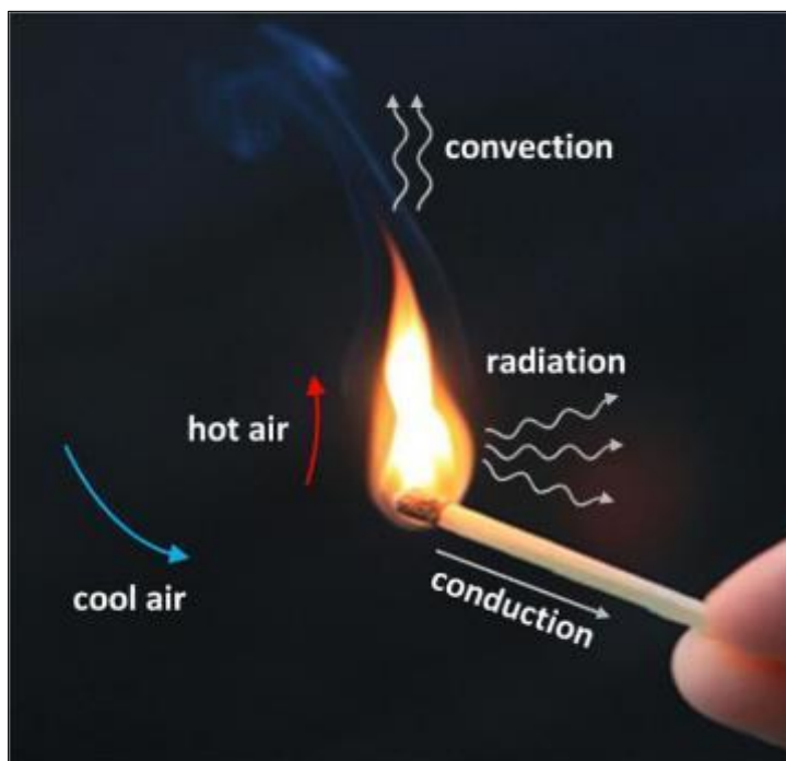
Figure 2 Basic mechanisms of heat transfer in a match flame adapted by “Flame Spread and Fire Behavior in a Corner Configuration
