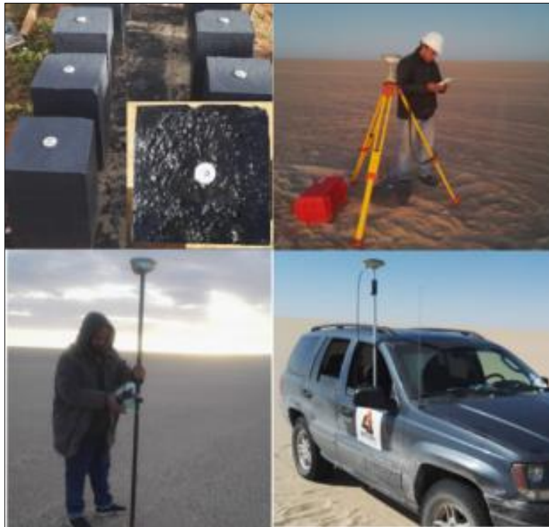
Figure 4 Fixing GCP's along the pipeline route using PPP, DGNSS, and RTK
