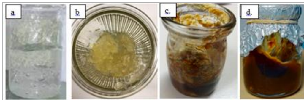
Figure 6 Color Change of Hydrogel Carrier During the Sterilization Process, Formulation, and Shelf Life of 126 Days. a.) non-sterile gel, b.) sterile gel, c.) biofertilizer with a shelf life of 0 days, d.) biofertilizer with a shelf life of 126 days
